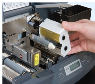
Special cleaning cassette easy to remove
