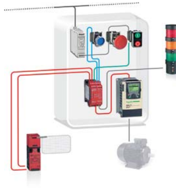
Safe stop 1 (PL d, SIL 2) Variable speed drive
