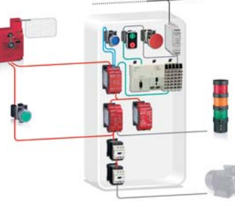
Zero speed detection (PL e, SIL 3)
