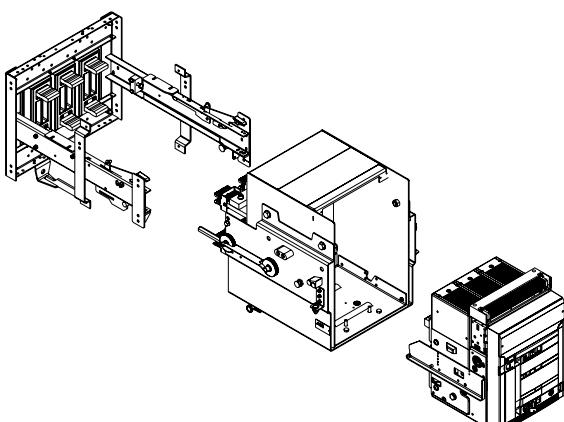
**Cradle in Cradle (CiC):** the fixed part of the new circuit-breaker is suitably adapted and tested in ABB. This solution allows the new fixed part be fast fitted inside the existing fixed part.
