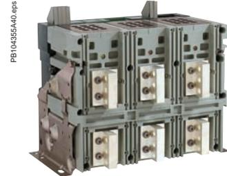
Simply turn a horizontal rear connector 90° to make it a vertical connector. For the 6300 A circuit breaker, only vertical connection is available.
