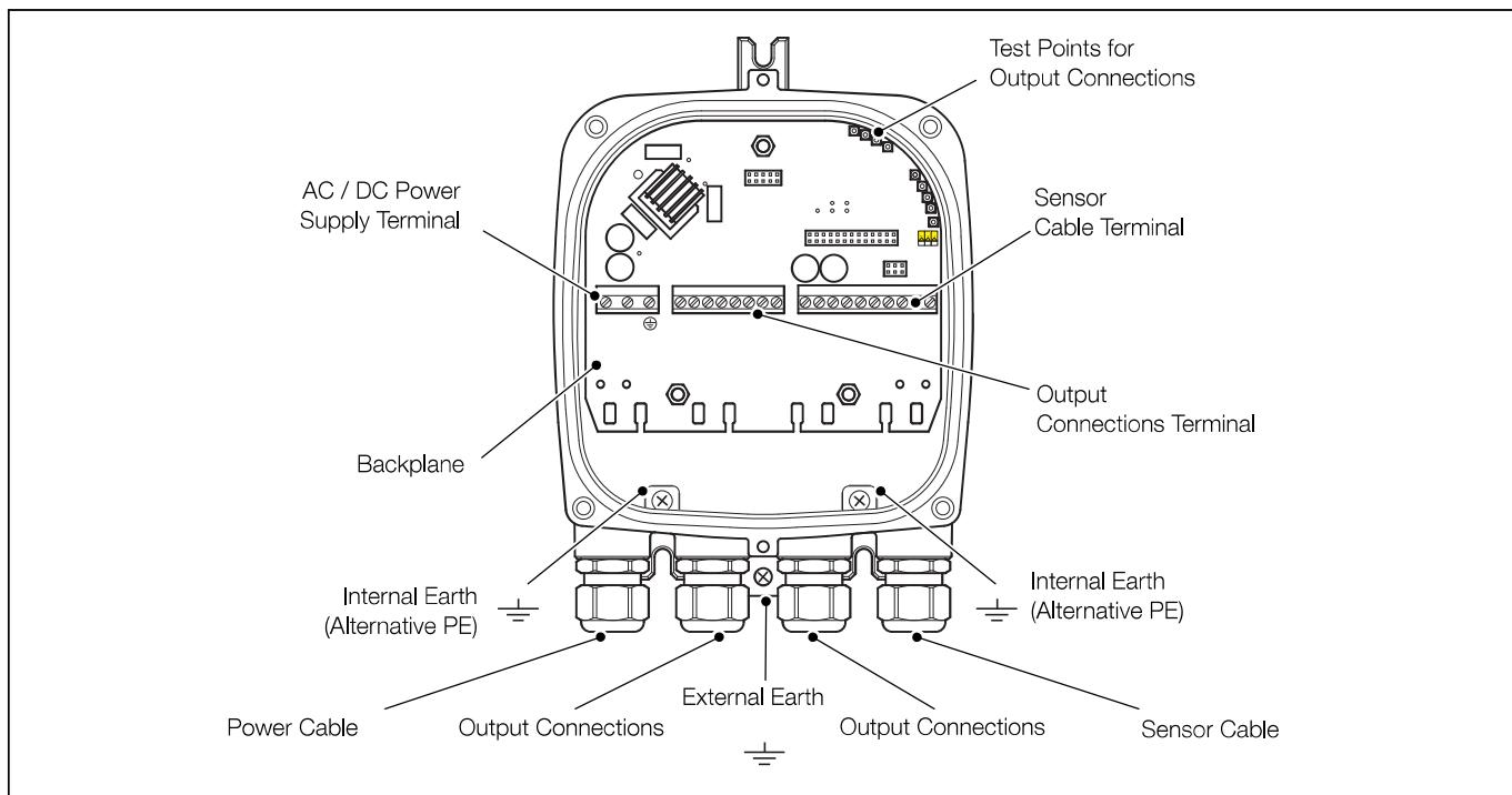
Cable gland / conduit entry (Remote transmitter shown)
