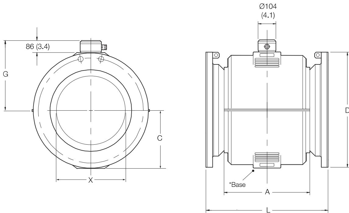
\*Dimension C = centre line to base of flowmeter body
