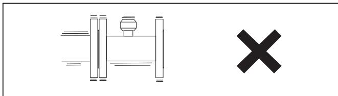
The flowmeter must not be submitted to any localized heat during installation; take care to remember this is a measuring instrument.
