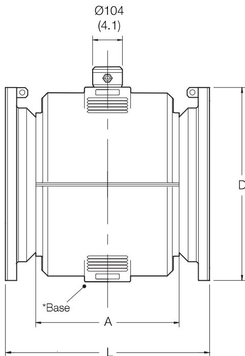
\*Dimension C = centre line to base of flowmeter body
