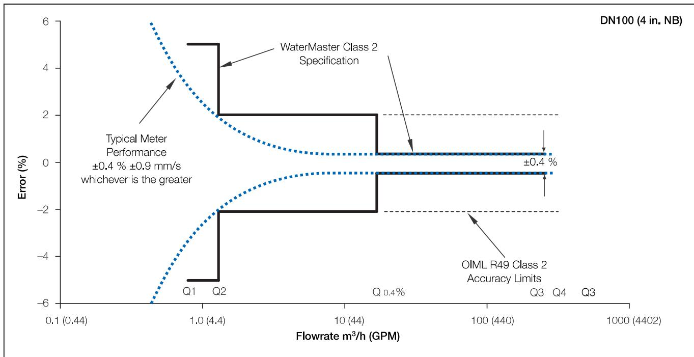
Although OIML R49 does not define the flow accuracy below Q1, WaterMaster continues to measure flow at lower flow rates down to a cutoff velocity of  $\pm 5$  mm/s ( $\pm 0.2$  in./s). The accuracy between cutoff and Q1 is typically  $\pm 0.9$  mm/s ( $\pm 0.04$  in./s).
