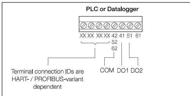
PLC / Datalogger connections
