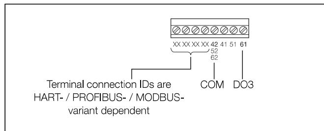
**Note.** Digital outputs DO1 and DO2 are polarity sensitive. The common (negative) connection for these outputs is designated 'COM'.
